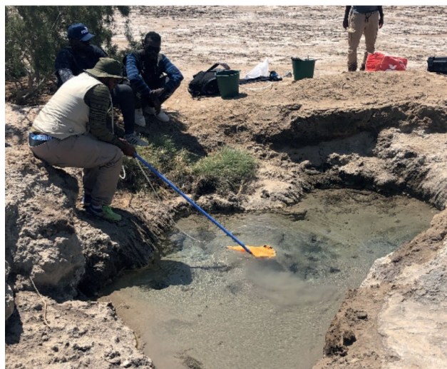
Figure 5 Gas sampling in a hot spring by geologists from ODDEG, CVA, GEO4U, UPPA and IFPEN, Lake Abbhé, Djibouti. Chromatographic and isotopic analysis shows the presence of hydrogen associated with helium of mantle origin (Rigollet et al., 2021).
