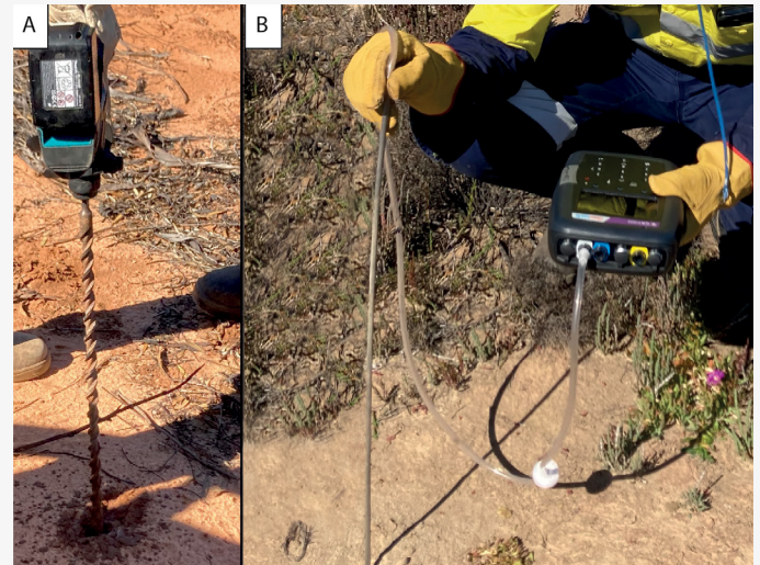
A. Handheld drill B. Handheld multi-gas analyser device
